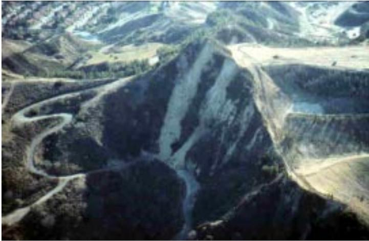
*Triggered by the Northridge earthquake of January 1994, twin landslides block a road near the I-5 interchange with California State Highway 14. Landslides, rock falls and rockslides in the Santa Susana and western San Gabriel Mountains blocked many roads and thus hampered relief efforts and exacerbated transportation problems caused by the earthquake. Courtesy, U.S. Geological Survey.*
