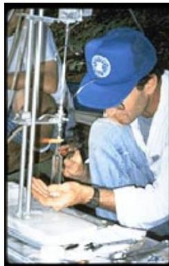
*A hydrologist testing for chlorofluorocarbons (CFCs), collects groundwater samples in a glass tube. Because exposure to air would contaminate the sample, he uses a flame to melt and seal the tube. Courtesy, U.S. Geological Survey.*
